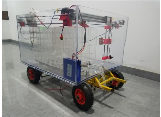
**Figure 7: Prototype of the self-driving concept express delivery vehicle**
