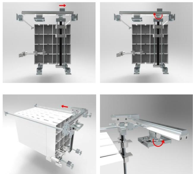
Figure 3: working process of the shelf moving mechanism
