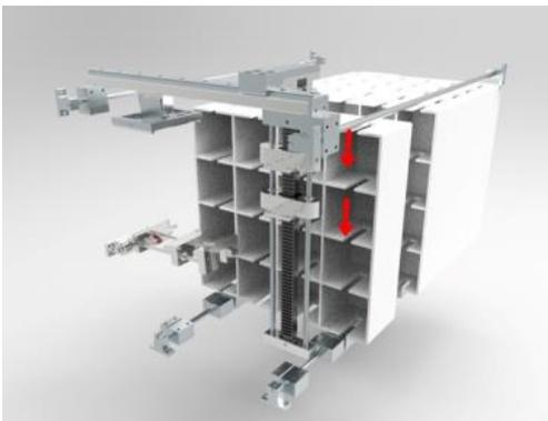
Figure 4: grabbing mechanism
