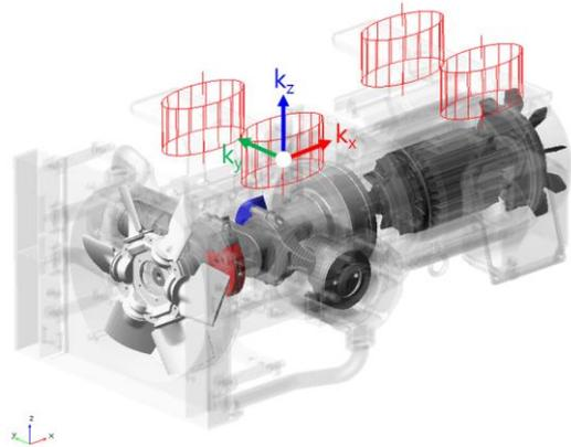
**Figure 4: The air compressor model in multibody dynamics program, MSC Adams.**
