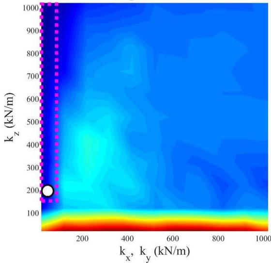
Figure 6: The motion of the air compressor motion with respect to mounting rubber stiffness.
