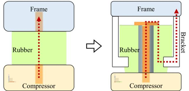
Figure 8: The original mounting rubber location(left) and the modified one(right) (Red dotted line : the path of transfer force)
