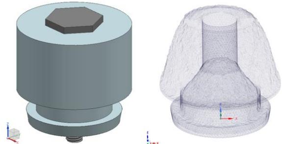
Figure 9: The mounting rubber with modified assembly method(left), Shape of proposed mounting rubber suggested by the second topology optimization(right)
