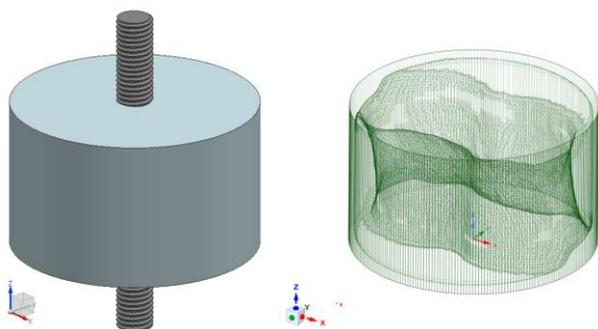
Figure 7: The shape of the baseline mounting rubber(left), The suggested design shape of the mounting rubber(right)
