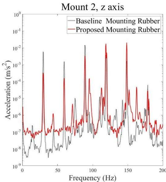
Figure 12: Acceleration magnitudes in frequency domain at point 2 (Black dotted line : The baseline mounting rubber case, Red line : The proposed mounting rubber case).
