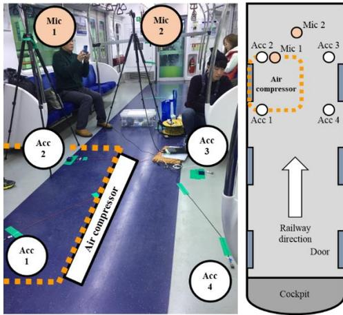
**Figure 2: Vibration and noise experiments carried out in running railway vehicles.**
