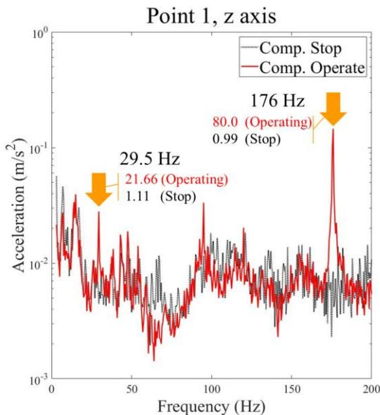
**Figure 3: The acceleration magnitude at the location of accelerometer 1 in the frequency domain depending on air compressor operation. (Grey line: The compressor is activated. Red line: The compressor stopped.)**
