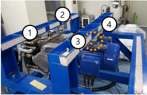
Figure 10: The jig test of the air compressor mounted at four points on the frame. The orange-dotted circle shows the proposed mounting rubber.
