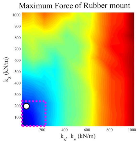
**Figure 5: Transfer force from the air compressor to frame with respect to mounting rubber stiffness.**
