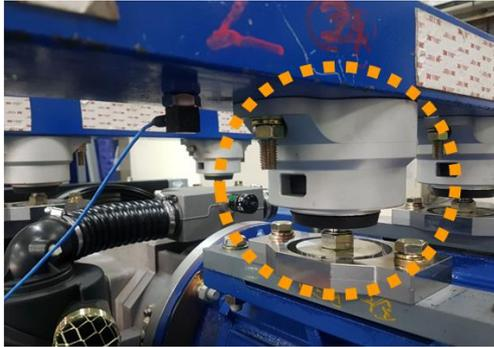
Figure 11: The picture of enlarged mounting rubber on jig with the force sensor on the bottom.
