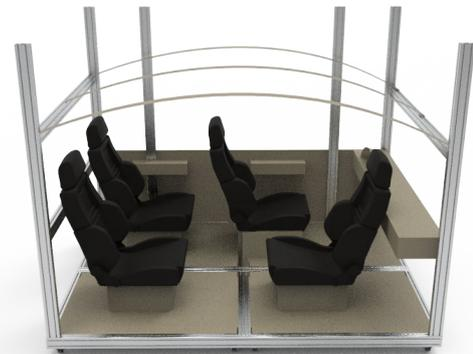
**Figure 4 :** Vehicle interior buck rendering
