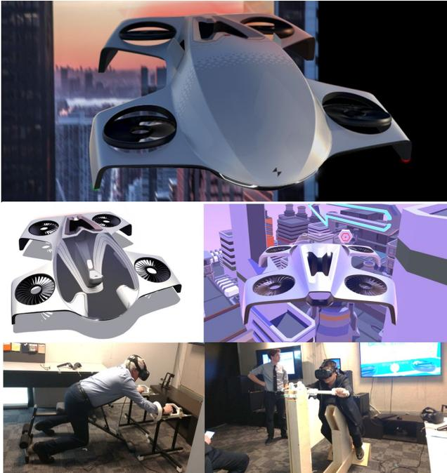
**Figure 5 :** Transportation Design 1 projects: Hunter Elmore’s high-fidelity CAD model (top and mid-left), and low-fidelity physical mock-up (bottom-left). Matt Whitby’s playable simulation (mid-right), and physical mock-up (bottom-right).
